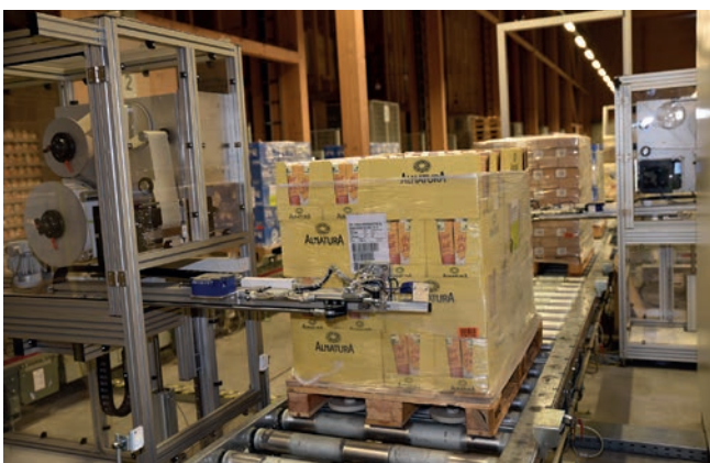
Pallet labeling at various heights
