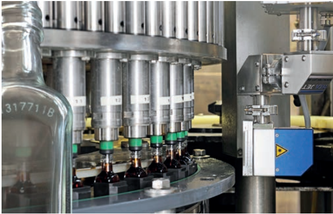
CL laser integrated into a bottling system (glass marking)
