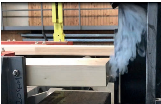
CL laser integrated into a wood processing center
