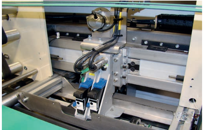
HR pro OEM integrated into an envelope-filling machine
