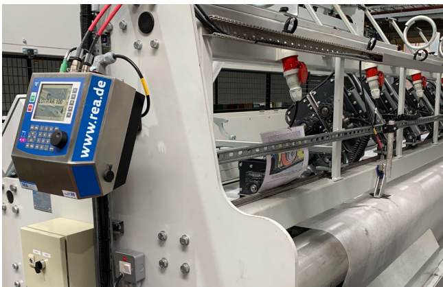
Marking of mesh material
