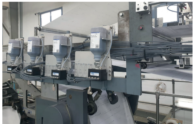
Bulk systems in large printing plant
