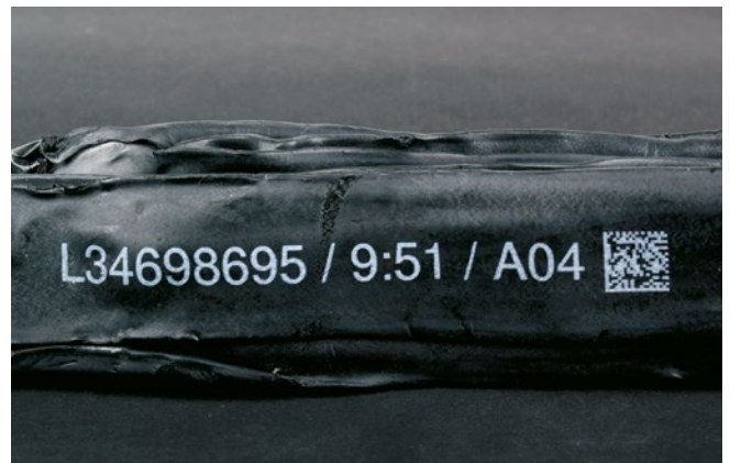
2D code on non-vulcanized rubber, printed with large character ink jet system
